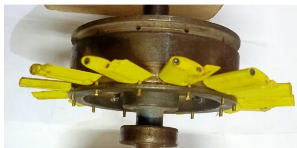
▪ Fig (6). Wells turbine model with small pins responsible for tail position.
