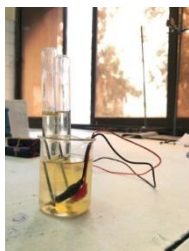
Fig (3): Electrolysis of water to produce green hydrogen gas.
