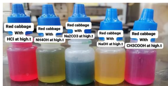
Figure (13): Red cabbage color in acidic and basic media at high temperature
