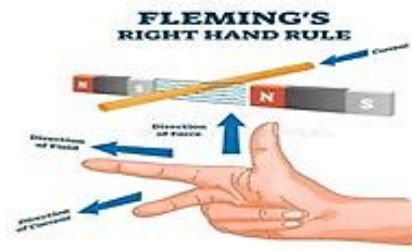
Figure (13) Fleming's right-hand rule.
