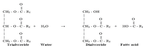
Fig. 3: Hydrolysis of triglycerides to form free fatty acid.
