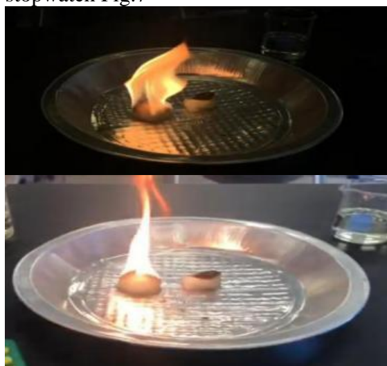
Fig.7.UCO stopped burning at 30 minutes and biodiesel stopped burning at 9 minutes.
