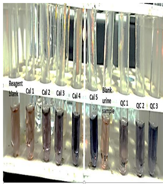
Figure (3). Gradient of blue colour complex in Meth spiked samples for calibrators and quality controls (Cal: calibrator, Qc: quality control).
