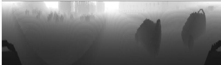
Figure 3 : "Depth value connected smoothly after correction" (show the before and after effect of the depth correction).
