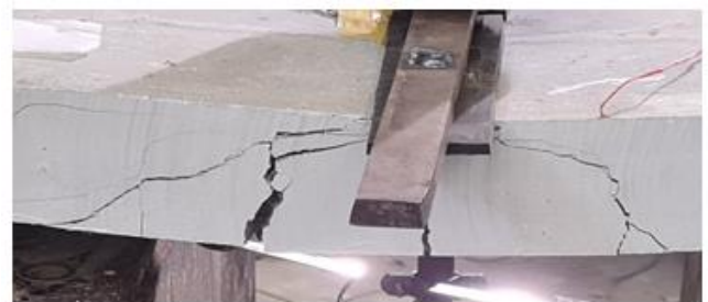
Figure 7. Fibers effect as bridging elements resisting crack propagation.
