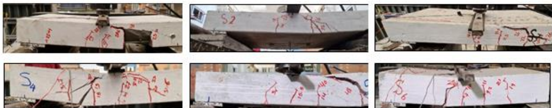
Figure 3. Flexural failure mode for slab specimens (S1 to S6).
