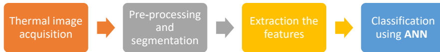
Fig. 2. The procedural framework for carrying out the core operations in the first proposed approach.
