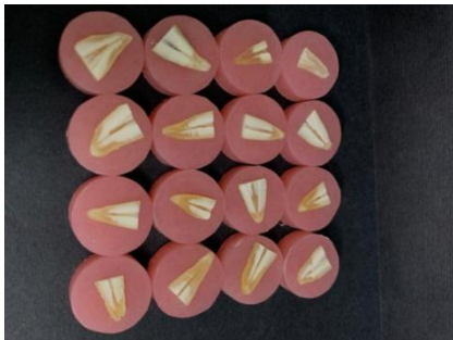
Fig. (2) Specimens mounted on acrylic blocks
