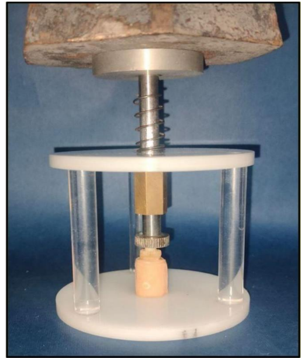
Figure 5 shows the specimens under the static load device
