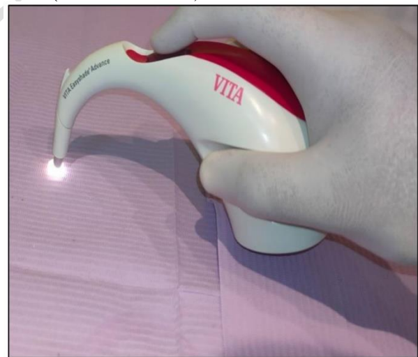
Figure 3 shows VITA EasyShade device recording the L* 1 a* 1 b* 1 values
