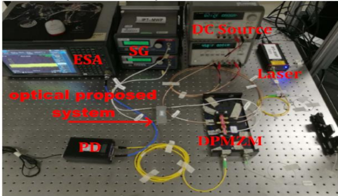
Figure 18. The experimental setup of test optical proposed system.
