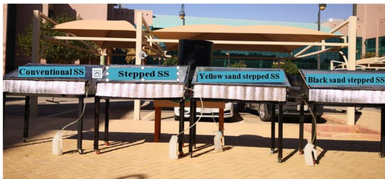
Figure 28. Photo of the experimental test rig [26].
