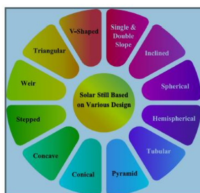
Figure 36. Classification of solar still based on geometry [32].
