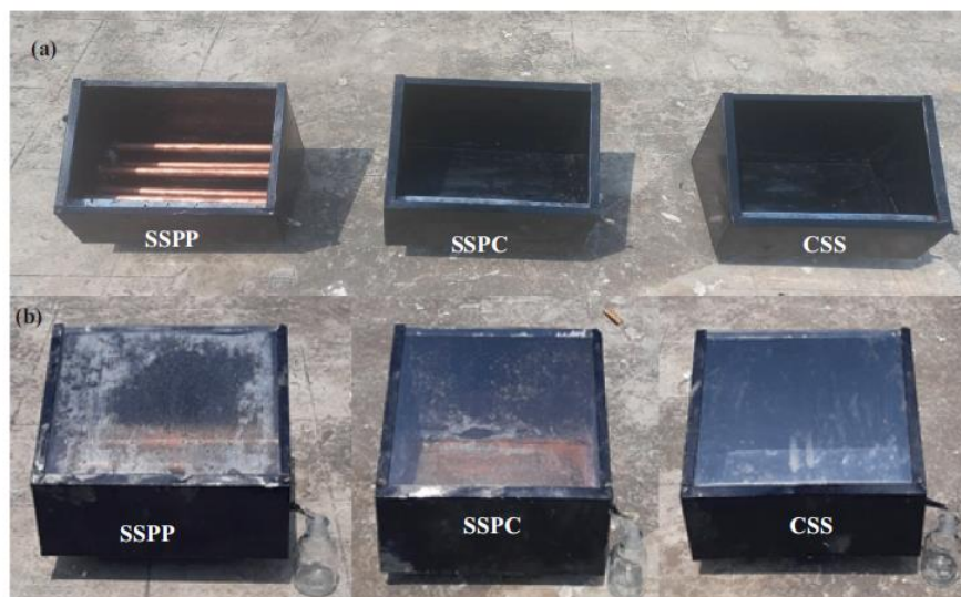
Figure 38. All three fabricated solar stills (a) Without glass cover and (b) With Glass cover [33].
