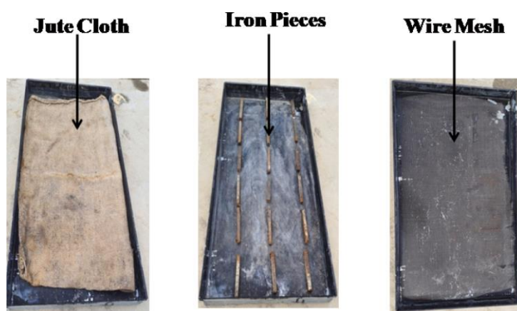
Figure 4. TSS with various energy-storing materials(a) Jute cloth, (b) Iron pieces, and (c) Wire mesh [5].
