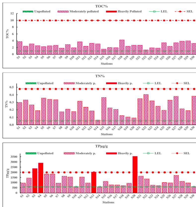
Fig.5. TOC%, TN% and TP \mu\text{g/g} in the studied sediment samples and their corresponding LEL and SEL concentrations values
