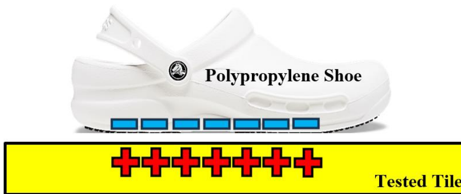
Fig.12 Illustration of the distribution of ESC on the sliding surfaces of PP shoe and the tested tile.
