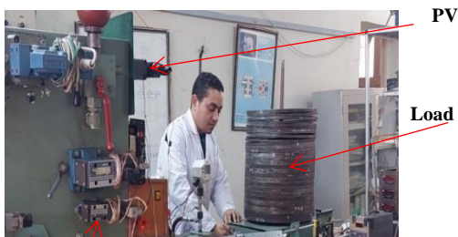
Fig. 4 Front photograph of the linear hydraulic system linear under experiments; system under loading
