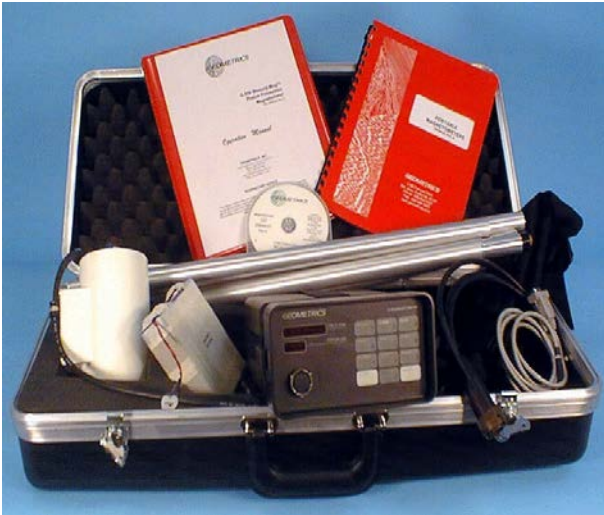
Figure 5a: G-856 Proton-Precession Magnetometer (Geometrics, 2010).
