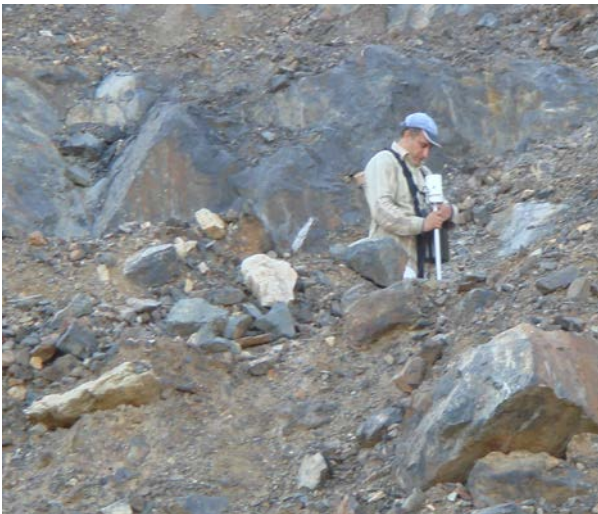
Figure 5b: magnetometer assembled & magnetic Data Acquisition in the studied area.
