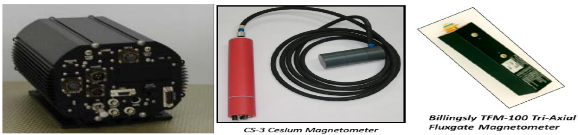
Fig. (2) : MMS-4 High-sensitivity magnetometer processor with its CS-3 sensor, and Billingsly TFM Tri-axial fluxgate magnetometer.
