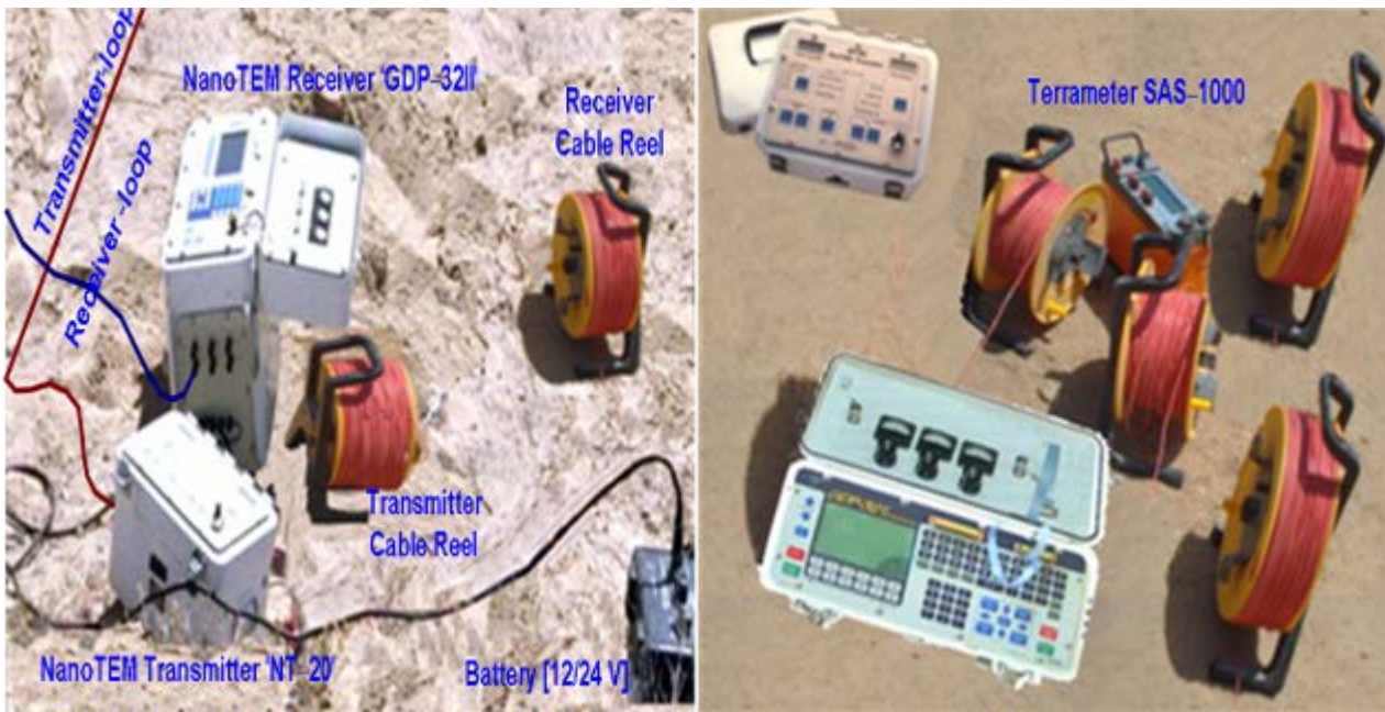
Fig. (2): Photographs showing both (left) the Zonge ® NanoTEM and (right) ABEM ™ Terrameter SAS-1000 measuring systems and other connections in the field.
