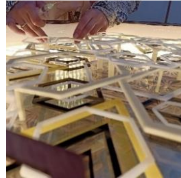
The stage of assembling the working parts using chloroform welding the eighth work
