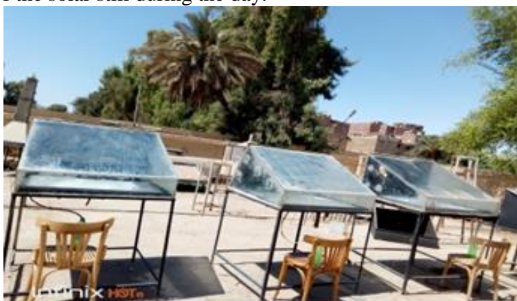
Fig. 1: Photo of the solar stills used
