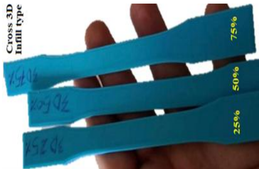
Figure 5: The printed specimens with Cross 3D infill type with different percentages
