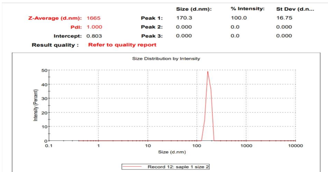
Fig 2: FEO-NE particle size was created using a 30-minute ultra-sonication process.
