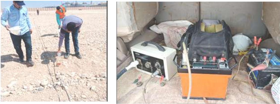
Fig. (4): The instrument SAS 1000 with multi-electrode system and field photo.
