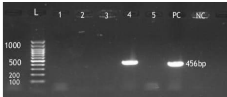
Fig. (1). PCR-assisted Agarose gel electrophoresis of the hlyA gene specific to L. monocytogenes : Lane L: Ladder, Lane 1-5: Isolates from various samples, Lane PC: positive control for hlyA at 456bp, Lane NC: negative control.
