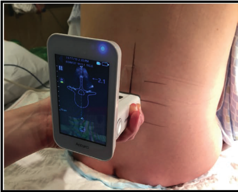
Figure 2. The wireless handheld ultrasound (Accuro, Rivanna medical, Charlottesville, VA) device investigated. The device has integrated software algorithm to depict bony landmarks and measure depth to spinous process and epidural space in real time. The image was downloaded from https://rivannamedical.com .
