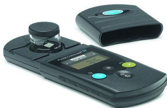
Figure 2: Portable Pocket colorimeter II used for analysis of fluoride concentration.
