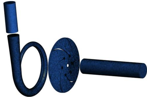
Fig. 3: Grid generation for the computational domain
