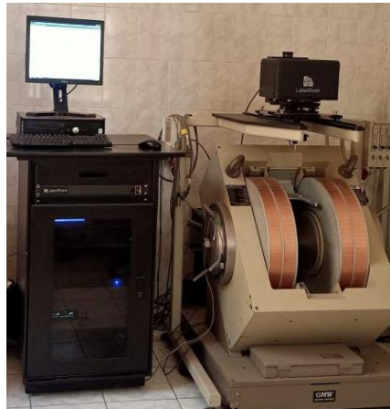
Fig. 1. Vibrating Sample Magnetometer apparatus
