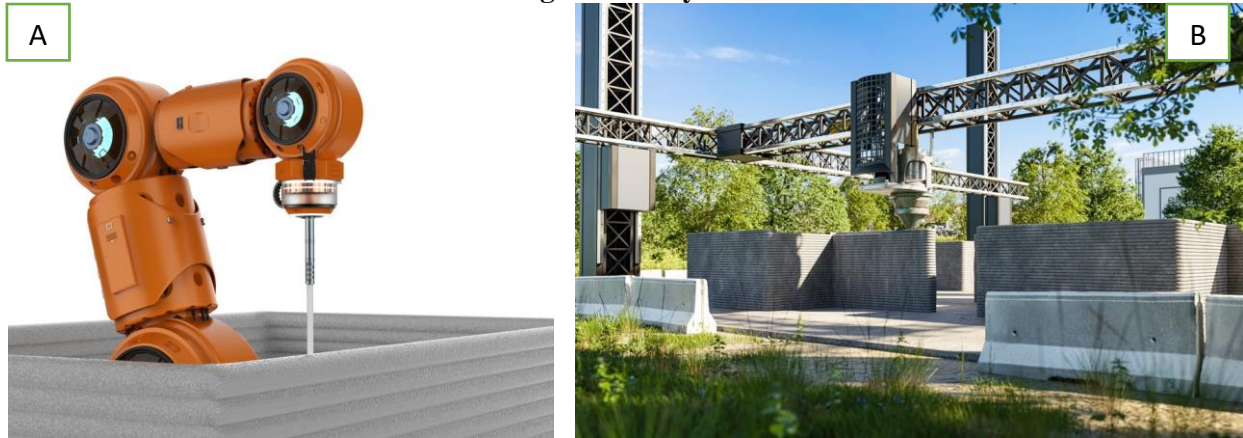
Fig. 3. (A) Robotic Arm Extruders; (B) Gantry System source [8].
