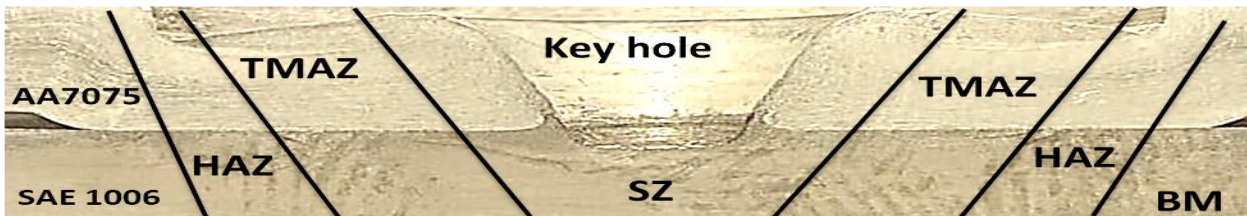
Fig. 3. Zones in FSSW composed of the Stir Zone (SZ), Thermo-mechanically Affected Zone (TMAZ), Heat Affected Zone (HAZ) and Base Metal BM) at 17 sec and short pin length.
