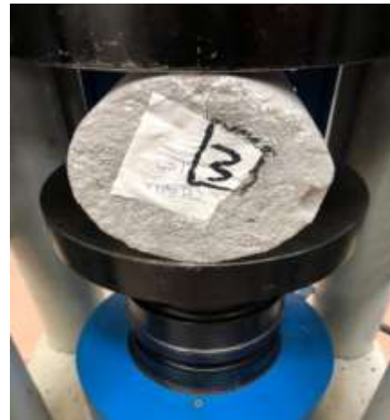
Fig. 6. Indirect Tension Test
