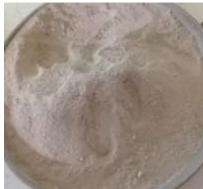
Fig. 3. Sample form of calcined clay produced by Asfour factory, Egypt
