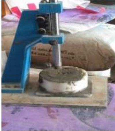
Fig. 1. Initial setting time test for Portland cement
