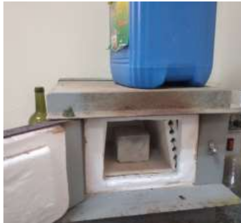
Fig. (7) Standard cube in electric furnace
