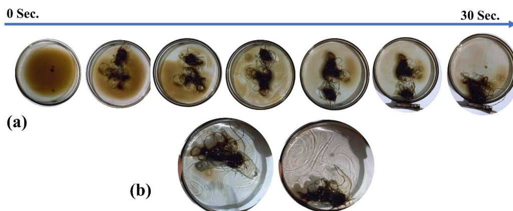
Figure 7 illustrates the efficient and controllable oil adsorption capabilities of (Par/St)CoFe 2 O 4 magnetized fibril wax in a waste engine oil-water mixture.
