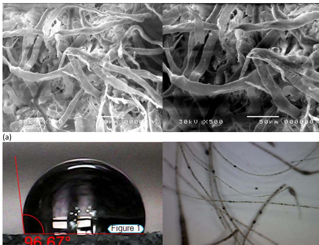
(a) Figure 6. The SEM image of (Par/St)/CoFe 2 O 4 magnetized fibril wax (a) and (b) contact angle with ( \theta = 96.67^\circ ) The left picture shows the microscope picture of (Par/St)/CoFe 2 O 4 magnetized fibril wax .
