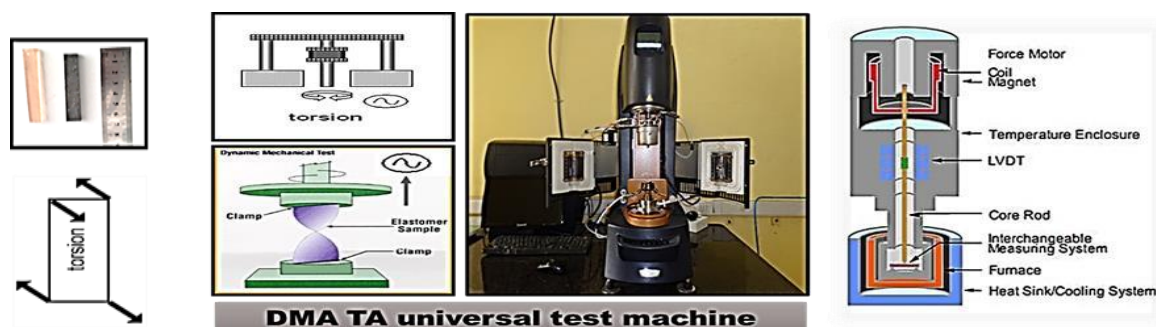
Figure 2. Dynamic mechanical analyzer and tested samples
