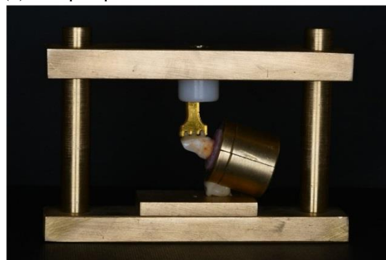
Figure (2): Specially designed static loading device used to holding the specimens and apply a static load during micro-disc cementation.
