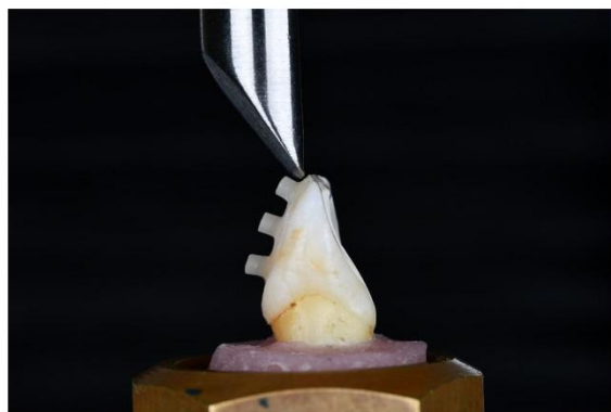
Figure (3): Mono-beveled chisel tip fell at the tooth and micro-disc interface.
