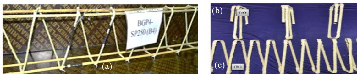
Figure 10. (a) GFRP reinforcement (b) individual rectangular GFRP(c) spiral stirrup GFRP.[9]
