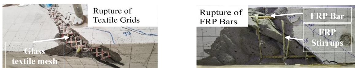
Figure 9. Failures of beams in the FRP.[1]
