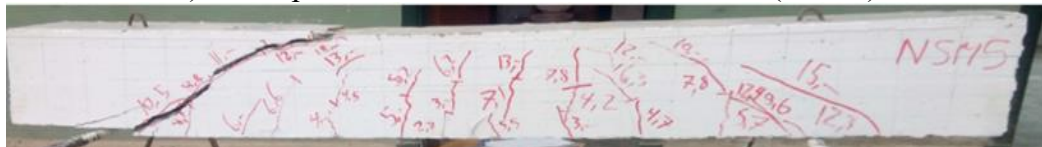
c) Crack pattern and mode of failure for beam (NSM5).
