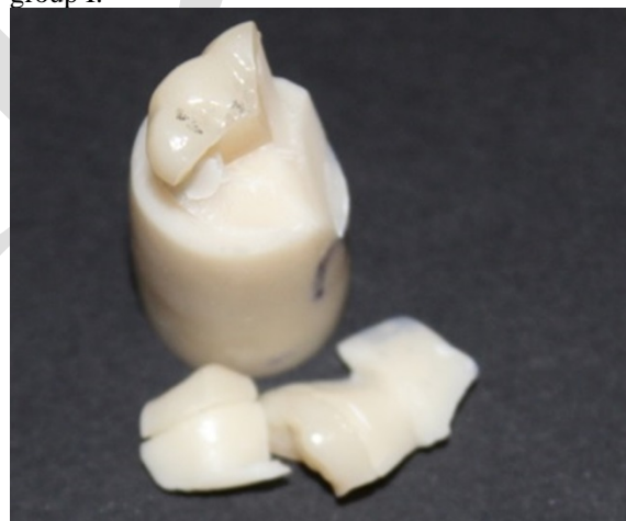
Figure (5): Class V mode of failure (40%) from group II.
