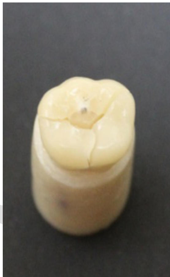
Figure (4): Class I mode of failure (20%) from group I.
