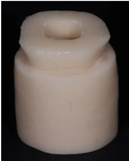
Figure (2): Epoxy resin die.
