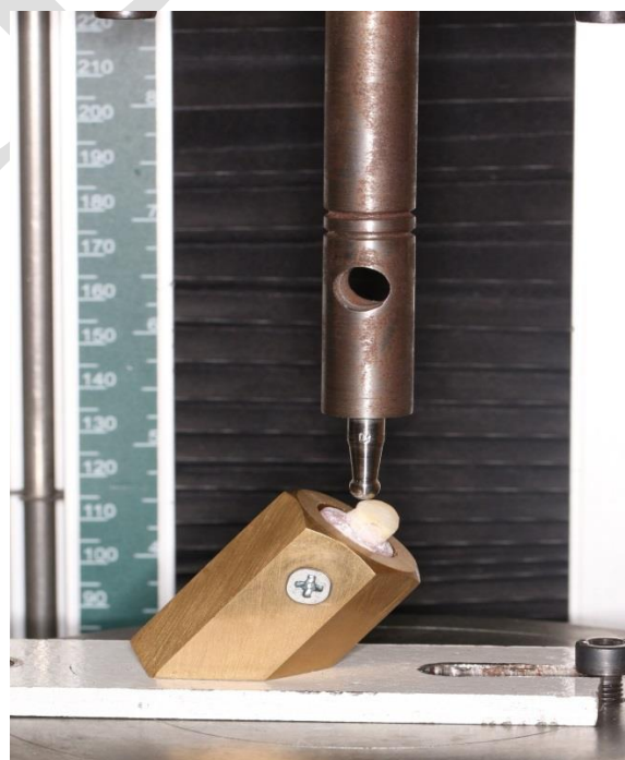
Figure (3): Showing specimen under universal test device.
