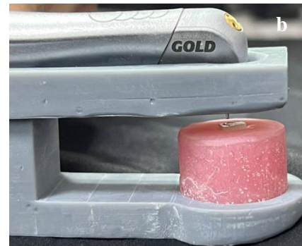
Figure (2): Custom-made 3D-printed holders designed to standardize the specified standoff distances during sandblasting (a), and laser surface treatments (b).
