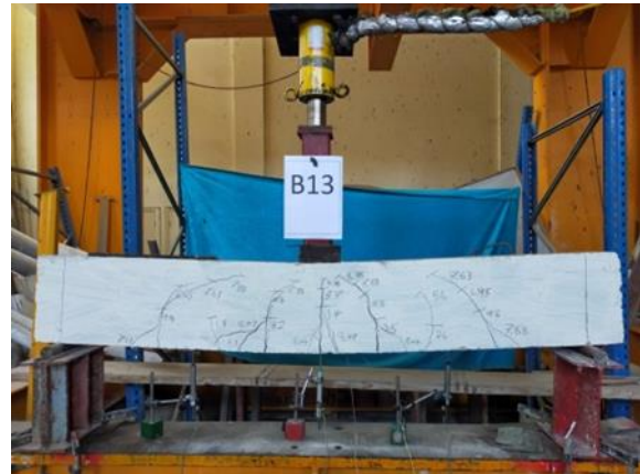
Fig 21. Crack pattern for B13.
