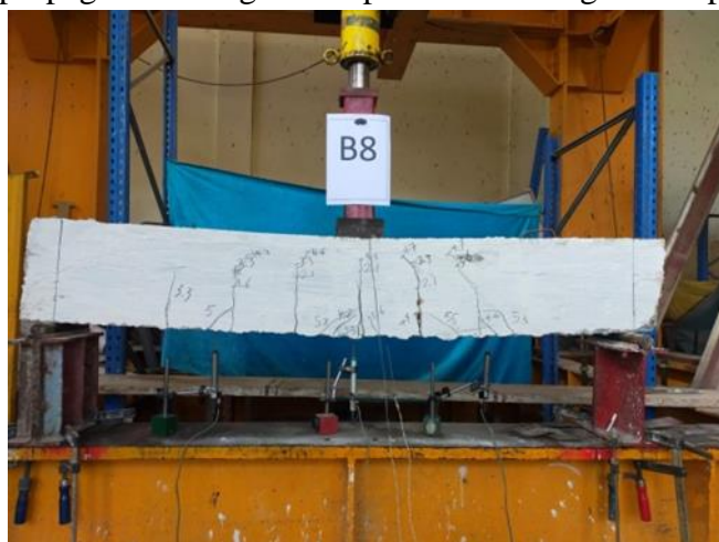
Fig 14. Crack pattern for B8.
