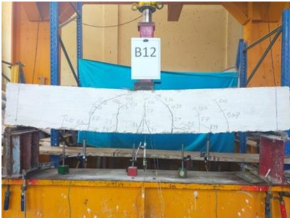
Fig 20. Crack pattern for B12.
