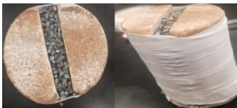
Fig. 6: The Oligocene sandstone platens with proppant before conducting fracture conductivity test.
