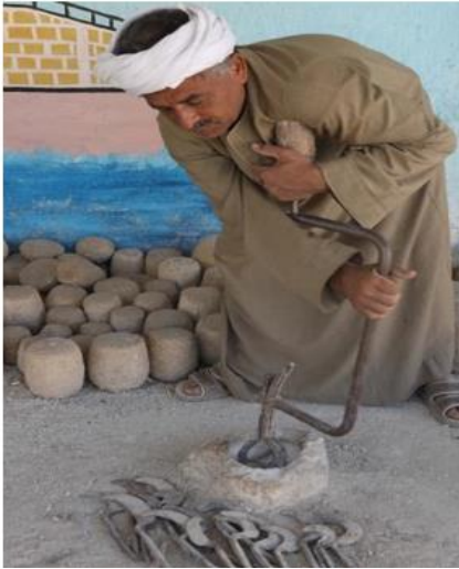
Fig. 18. Stoneworker using a drill with a special crank to hollow out a stone vessel (photo taken by the researcher, October 10, 2021).
