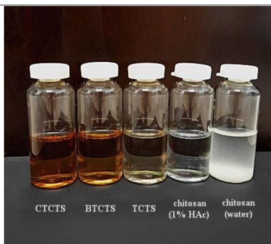
Figure 2. Different produced solutions of the designed chitosan derivatives prepared in neutral water at a concentration of 1.0 mg/mL, alongside a chitosan solution in neutral water supplemented with 1% acetic acid (HAC) [62].
