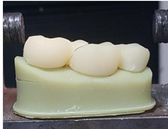
Figure (2): CAD/CAM IFDP Mode of Failure (premolar-molar connector).
