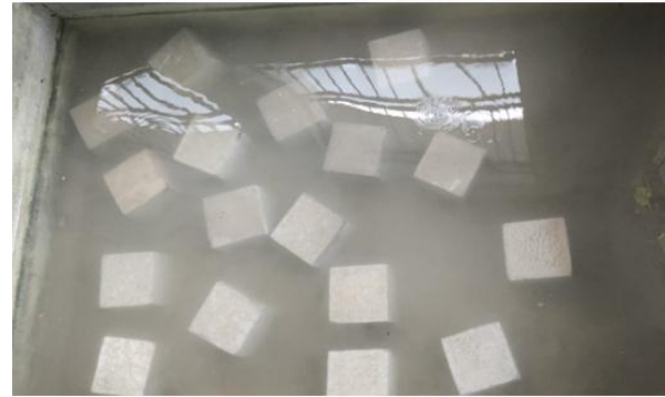
Figure 4: Curing of Concrete Cubes
