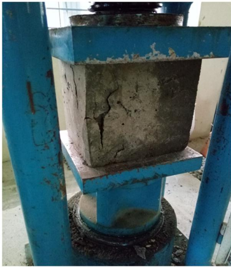
Figure 5: Broken Specimen after Reach Ultimate Load
