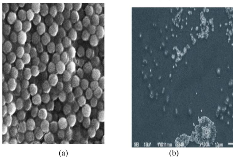
**Fig 4. Figure 4a Result of Scanning Electron Microscopy Biofilm with No Treatment, Figure 4b Result of Scanning Electron Microscopy Biofilm with administration of kratom extract 30% b/v.**
